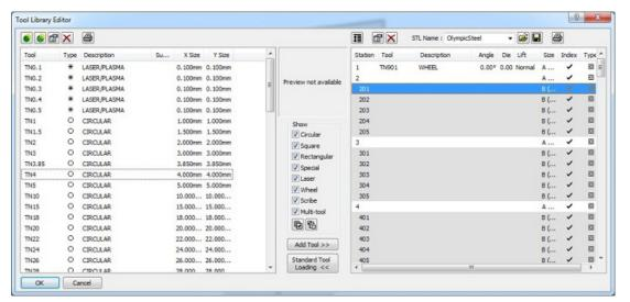
Conversely, if a tool is placed in a main turret station, the multi-tool positions are not shown (as can be seen in the image – station 1).
