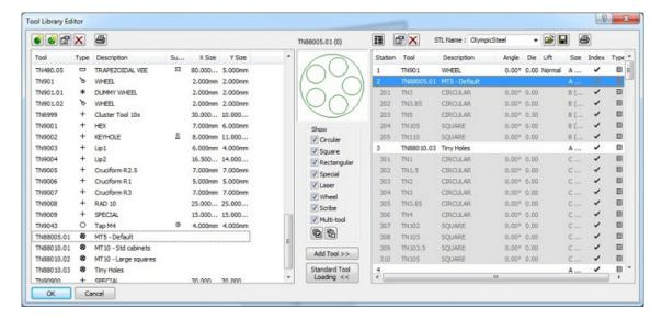
These pre-loaded multi-tools can be loaded into the (standard) turret, therefore loading all tools at once – they can also be moved to a different turret station as a whole.
